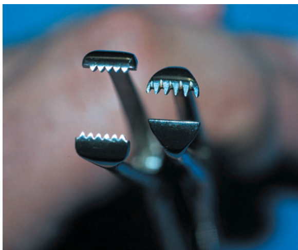
Fig. 1. (Left) The Allis forceps. (Right) Removing the teeth from one side of the Allis forceps and deepening those on the opposite side will create the Cabas-Coffler marker.
